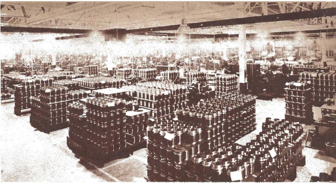
An idea of the magnitude of America's defense effort may be gained from this view showing thousands of steel cylinder barrels stacked row on row in a corner of the Paterson factory of the Wright Corporation, the nation's largest aircraft engine manufacturing organization.
