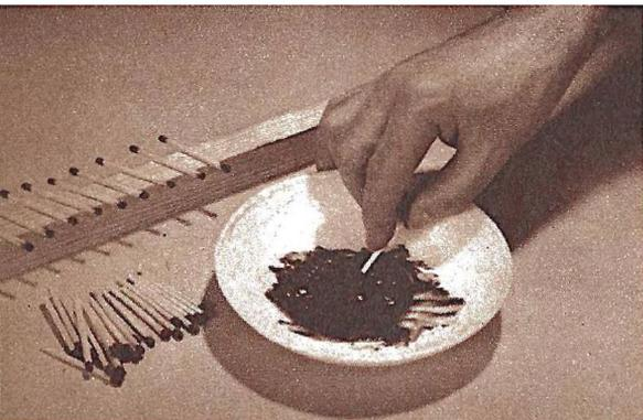
Coating the ends of safety matches with the igniting material so they can be lighted twice.
