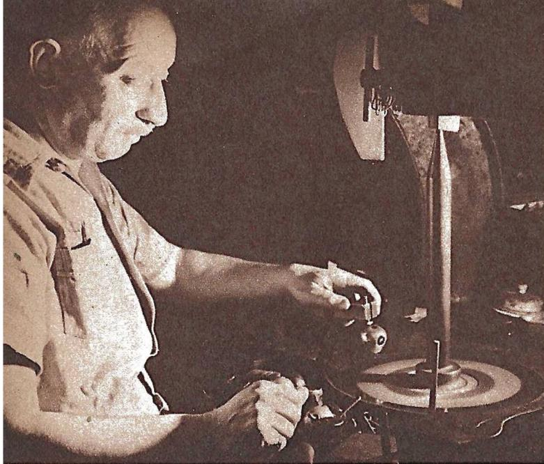
Left: Set in the "dop," a cut diamond is placed on the polishing wheel, which is treated with diamond dust and oil.
