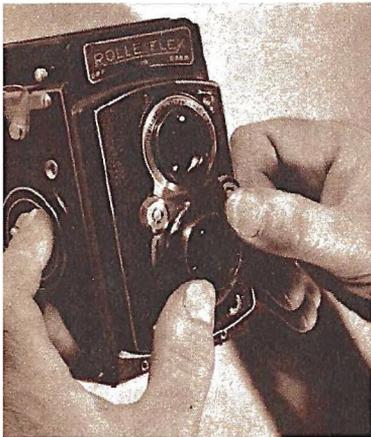
Above: Cellophane held taut in front of the camera lens serves as a filter. The material must be held flat to avoid lens flare and distortion. Place a square of cellophane over the lens; then, press over it a ring of brass tubing which normally fits lens mount loosely.—*Kenneth Murray.*
